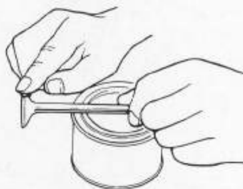
Fig. 3-5-18 Applying lapping compound to valve face
