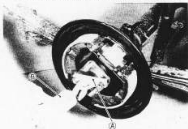
Fig. 17-2-7 Ⓐ Special Tool (Rear Axle Remover 09922-66010) Ⓑ Special Tool (Sliding Hammer 09942-15510)
