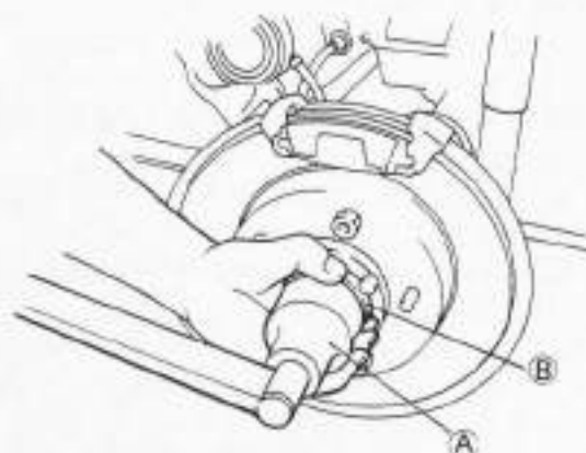
Fig. 17-5-23 Special Tool (A) (Front Wheel Bearing Nut Socket Wrench 09941-58010) Special Tool (B) (Automatic Free Wheeling Hub Socket 09944-98010)
